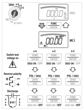
Starting the insulation resistance measurement: Briefly press the Uiso ON / OFF key.
